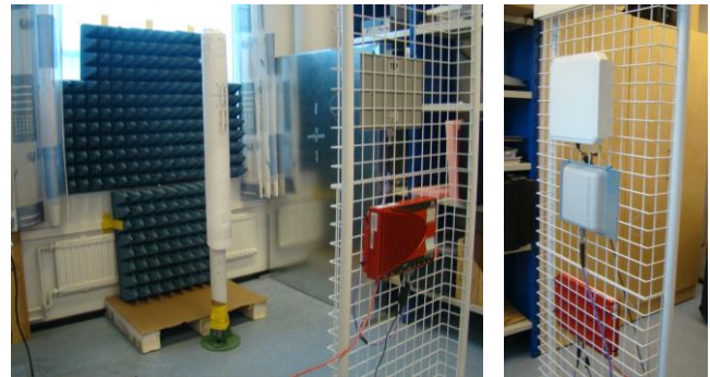
Fig. 5. The measurement setup. Tags are attached on the styrofoam pillar and readers and antenna on the rack on right. Impinj reader at the bottom, antenna in the middle, and ThingMagic reader uppermost.
