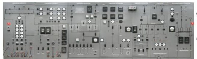
Figure 1: WVU power simulator in original configuration
