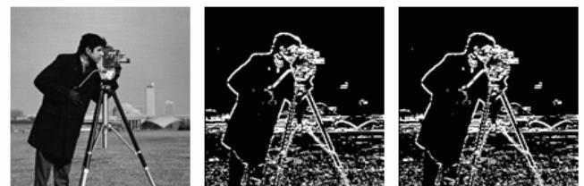
(a). Original image (b). Software (c). FPGA Figure 18. Comparison of edge detection by software and FPGA
